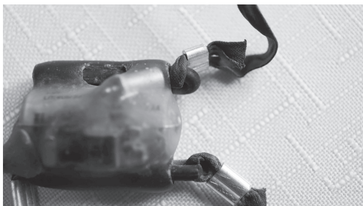
Figure 8 - Radio-transmitter type 1 – central tail feathers mounting method (photo: Christoph Leditznig).
